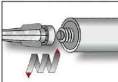
1. Remove the cap and attach the supplied static-mixing nozzle to the cartridge and load the cartridge into the correct dispensing tool. Cut off the foil tube clip before use. For every working interruption longer than the recommended working time (Table B3) as well as for new cartridges, a new static-mixer shall be used.
