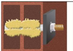
9. After full curing, the fixture can be installed with the max. torque (Table B2) by using a calibrated torque wrench.
