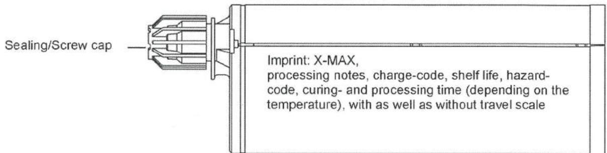
165 ml and 300 ml cartridge (Type: "foil tube")
