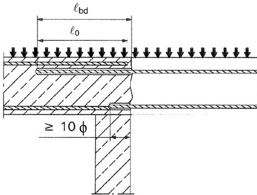
**Figure A2:** Overlapping joint at a foundation of a wall or column where the rebars are stressed in tension
