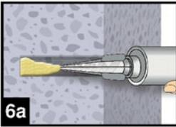
6. Starting from the bottom or back of the cleaned anchor hole fill the hole up to approximately two-thirds with adhesive. Slowly withdraw the static mixing nozzle as the hole fills to avoid creating air pockets. For embedment larger than 190 mm an extension nozzle shall be used.
