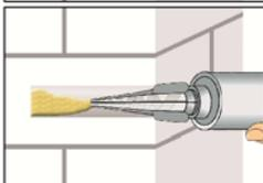
5. Starting from the bottom or back of the cleaned anchor hole fill the hole up to min two-thirds with adhesive. Slowly withdraw the static mixing nozzle as the hole fills to avoid creating air pockets. Observe the gel-/ working times given in Table B3.
