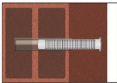
5. Insert the perforated sleeve into the bore hole. Make sure that the sleeve fits well into the hole. Never cut the sleeve! Only use sleeves that have the right length.
