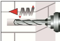
3. Holes to be drilled perpendicular to the surface of the base material by using a hard-metal tipped hammer drill bit. Drill a hole, by rotary drill mode, into the base material, with nominal drill hole diameter and bore hole depth acc. to the size and embedment depth required by the selected anchor. In case of aborted drill hole the drill hole shall be filled with mortar.
