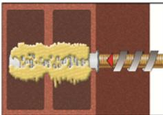
7. The position of the embedment depth shall be marked on the threaded rod. Push the threaded rod into the anchor hole while turning slightly to ensure positive distribution of the adhesive until the embedment depth is reached. The anchor should be free of dirt, grease, oil or other foreign material.
