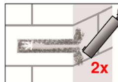
4. Blow from the bottom of the bore hole two times. Brush the hole clean two times, and finally blow out the hole again two times.
