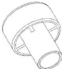
**Piston plug for overhead or horizontal installation**
