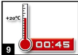
9. Observe gelling time  $t_{gel}$ . Attend that the gelling time can vary according to the base material temperature (see Table B3). It is not allowed to move the bar after gelling time  $t_{gel}$  has elapsed. Allow the adhesive to cure to the specified time prior to applying any load. Do not move or load the bar until it is fully cured (attend Table B3). After full curing time  $t_{cure}$  has elapsed, the add-on part can be installed.
