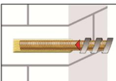
6. The position of the embedment depth shall be marked on the threaded rod. Push the threaded rod into the anchor hole while turning slightly to ensure positive distribution of the adhesive until the embedment depth is reached. The anchor should be free of dirt, grease, oil or other foreign material.
