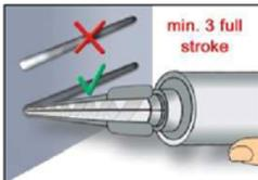
2. Place in the cartridge to an appropriate dispenser tool. Prior to dispensing into the anchor hole, squeeze out separately a minimum of three full strokes and discard non-uniformly mixed adhesive components until the mortar shows a consistent grey colour.
