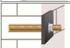
9. After full curing, the fixture can be installed with the max. torque (Table B1 or B2) by using a calibrated torque wrench.
