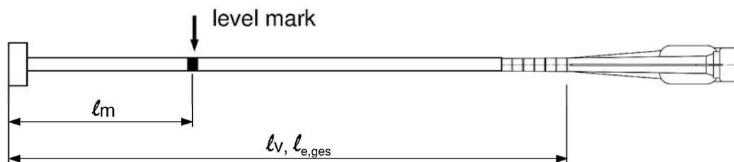
Injection tool must be marked by mortar level mark  $l_m$  and anchorage depth  $l_v$  resp.  $l_{e,ges}$  with tape or marker.
