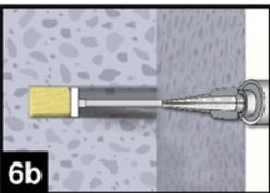
For overhead and horizontal installation and bore holes deeper than 240 mm a piston plug and the appropriate mixer extension must be used.
