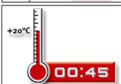
8. Allow the adhesive to cure to the specified curing time prior to applying any load or torque. Do not move or load the anchor until it is fully cured (attend Table B3).
