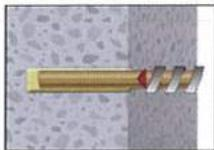
7. Push the threaded rod or reinforcing bar into the anchor hole while turning slightly to ensure positive distribution of the adhesive until the embedment depth is reached.
