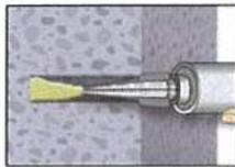
6. Starting from the bottom or back of the cleaned anchor hole fill the hole up to approximately two-thirds with adhesive. Slowly withdraw the static mixing nozzle as the hole fills to avoid creating air pockets. For embedment larger than 190 mm an extension nozzle shall be used. For overhead and horizontal installation a piston plug (Annex B 3) and extension nozzle shall be used. Observe the gel-/ working times given in Table B4.
