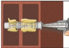
6. Starting from the bottom or back fill the sleeve completely with adhesive. For quantity of mortar attend cartridge label. Observe the gel-/ working times given in Table B3.
