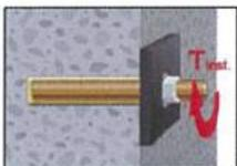
10. After full curing, the add-on part can be installed with the max. torque (Table B2) by using a calibrated torque wrench.
