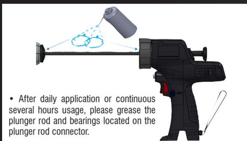
• After daily application or continuous several hours usage, please grease the plunger rod and bearings located on the plunger rod connector.
