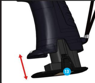
To remove the battery pack, press the battery release buttons and pull. **13**.
