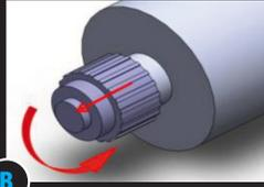
**B** Release and remove the coaxial cartridges cap.
