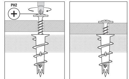
Insert the screw in the center of the plug and then, tight through the fixing piece
