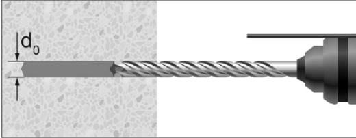
Drill the hole to the bore hole depth  $h_1$ .
