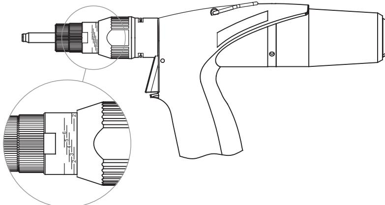
10. Adjust revolvable air supply into any required position and connect the tool to the source of the compressed air.
