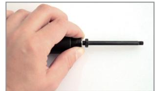
Unscrew the rod in place and screw in the rod corresponding to the diameter of the plug to be installed (M4 to M8). The cache snaps back into place. Then re-tighten the nose corresponding to the diameter of the rod used.
