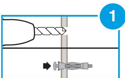
Drill the support to the specified diameter.
